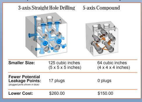
Sun's Custom Valvepaks are available in any configuration, limited only by the designer's imagination. Valvepaks reduce size and cost of hydraulic systems, take up less space, use fewer components, and have less potential leakage.
